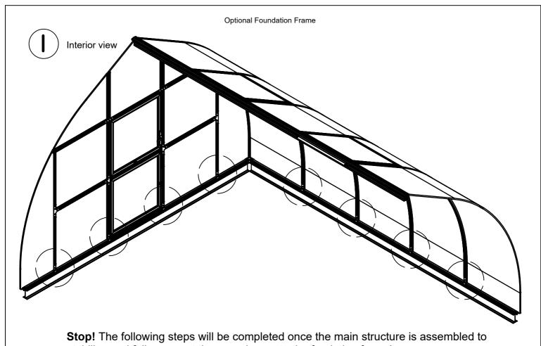
stabilize and fully connect the greenhouse to the foudation frame!
