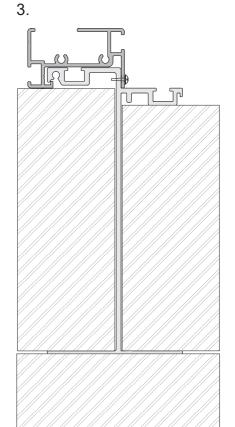
First hook the foundation frame into the soil profile, then rotate it into position.
