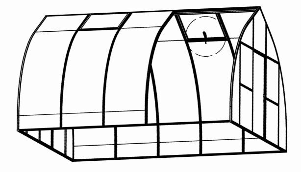
The Automatic Window Opener must be parallel to the roof window in order to open properly.
