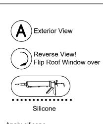
Apply silicone where the polycarbonate meets the metal profile and along the edge to prevent leaking.
