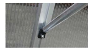
Attach strut to greenhouse curve with bolt (S5) and nut (S1). Tip: Insert bolt (S5) at the insertion point near the bottom of the curve. Please note that the black angle may not match the angle of your greenhouse curve.
