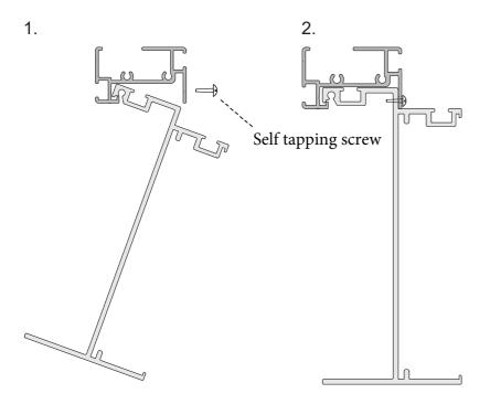
**Note:** Foundation frame profiles are shorter than the floor profiles!
