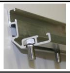
Insert one M6 x 12 bolt (S12) per curve of greenhouse (including the edge curves) into the lower channel on the bottom of the longitudinal profile (pos.1) of the shelf kit. Tip: Use a strip of tape to keep the bolts from sliding out the end.
