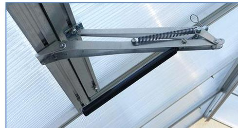
The opening temperature is controlled by the distance you thread the cylinder into the yoke. Fully threaded, the window will open at the minimum temperature. Thread the cylinder farther out (anti clockwise) to raise the opening temperature.
