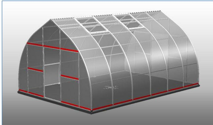
Seal the bottom edge of every glazing panel. Mask with Scotch Blue painter's tape to form a bead on the glazing surface 3 to 5 millimeters wide from the profile edges. Apply the sealant and tool it to slope from glazing surface to profile edge. Allow it to cure for 24 hours before removing the tape.
