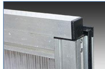
Install the seal in the door's top profile before you attach the rectangular tube. The seal material should extend over the full width of the door, not just the width of the rectangular tube. You can trim it after the door is fully assembled. The pre-drilled holes in the rectangular tube are offset, so it will fit only one way on the top profile.
