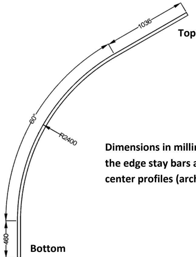
**Dimensions in millimeters of the edge stay bars and curved center profiles (arches).**
