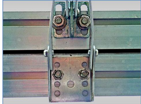
Chill the actuator in a refrigerator for about 10 minutes to assure that it is fully retracted. Manually press the shaft as far as it will go into the cylinder, and then fully thread the actuator into the yoke on the mechanism. Raise the window as needed to align the hole in the shaft with that of the bushing and install the locking pin. Finish by replacing the springs.
