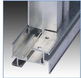
The curved vertical profiles of the side walls are fastened to the floor profiles and to the substrate by the mounting brackets (Pos. 6.7). The vertical profiles of the gable walls are initially fastened to the floor profiles with 4.2 by 13 mm self-tapping Phillips head screws and ultimately by mounting brackets.
