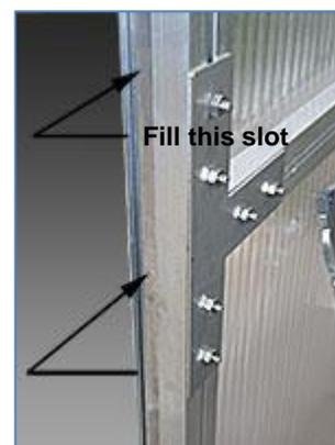
Install the lower screen first, then the upper screen. Or you can install the upper screen alone and close the lower door. Install an extra sash lock (Pos. 136) on the outside face of the left vertical door profile to keep the lower door closed when the upper door is open. Tape the screen to the vertical door profiles with Scotch Blue Painter's tape to keep it in place when the lower door is opened.
