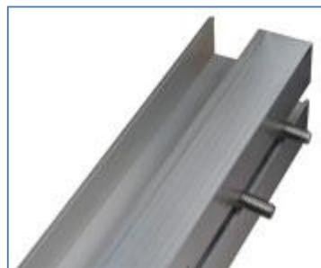
The M6 screws are loaded into capture slots in the various profile extrusions. All of these slots, and consequently all M6 screws, face the interior of the greenhouse. The M6 screws are loaded into the slots from the open ends and should therefore be loaded before the profile is secured in place. Loading a screw after the profile is in place is inconvenient and may require some disassembly.
