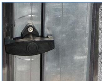
The spring side fits nicely in the deep door slot but it is helpful to partially fill the left door slot for a snug overall fit. Place an extra piece of the aluminum frame material into this slot to take up the slack. You should drill a hole in this filler to clear the head of the Phillips pan head screw (Pos. 142) that secures the crossbar to the vertical profile.
