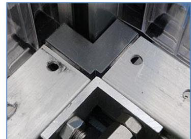
Fasten the cover in place when the holes are properly aligned. Then tighten the floor profile connector fasteners with a 10 mm socket. **You will not be able to tighten these fasteners if you loaded M6x16 screws in these positions.**
