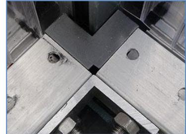
But with the cover in place a visual inspection reveals misalignment of the right-side holes. Because the floor profiles are tightly joined by the floor profile connector, an attempt to force the screws through the cover and into the floor profile on the right side would damage the screws and the profile.
