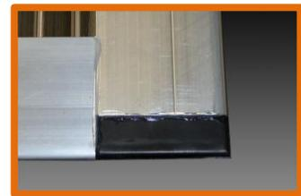
**Fasten the two side profiles to the bottom profile.** Use the provided 4.2 x 60 mm Phillips head screws. **Always drive the inner screw first** (marked 1 on the drawing) to pull and hold the profiles tightly together, then drive the outer screw (marked 2 on the drawing). The outer screw engages threads in the plastic corner connector before reaching the profile's screw channel and tends to jack the two profiles apart if not held tightly together by the first screw.
