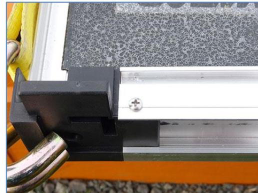
You must use the roof beam fitment tool to assure proper alignment of the arches before driving self-drilling screws.
