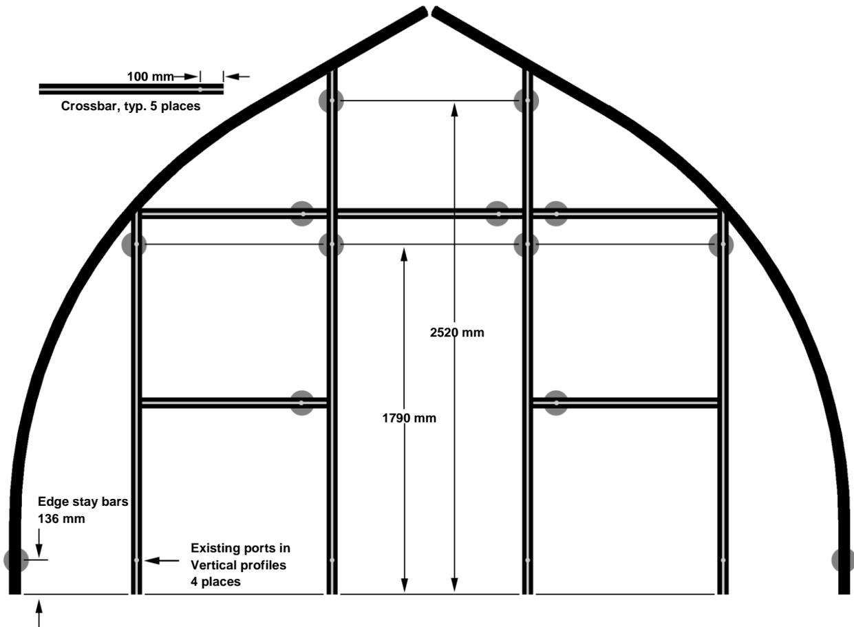
Cut the port with a small round file or a rotary file. Alternatively a pilot tool with a bore to guide a  $\frac{7}{16}$  inch end mill can be fabricated that will clamp onto a screw capture slot, retained by a cam-head screw.
