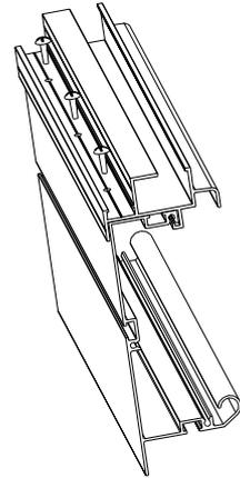
We recommend you permanently attach the Base sections to the Floor Profiles with Self Tapping metal screws – 3 screws in front and back and 5 screws on each side.
