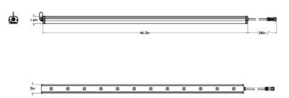
Fixture is designed to fit in 48" modules including all connectors and fittings
