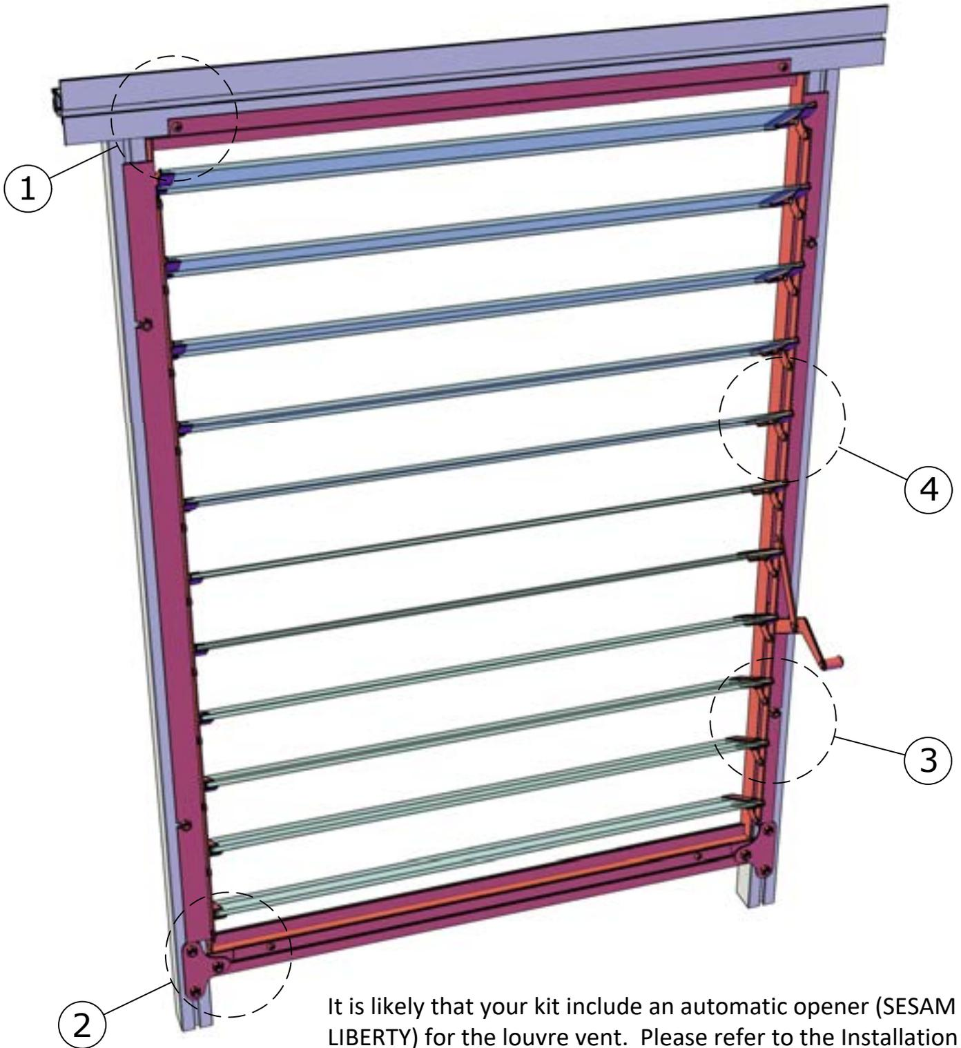
Insert a washer between black louvre frame and the greenhouse profile at all four bolt locations.
