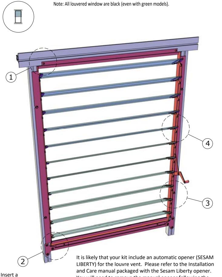
washer between black louvre frame and the greenhouse profile at all four bolt locations.
