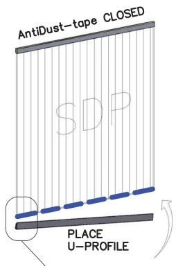
You will find a bundle of WHITE U profiles in the pallet. Place them over the vented tape. This will be the bottom of your polycarbonate panel. The U channel creates a space for any condensation to exit and move away from the panel. (white is the only available color)
