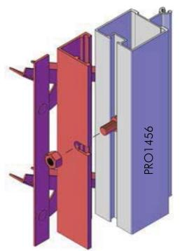
Insert a washer (not included) between black louvre frame and the greenhouse profile at all four bolt locations.
