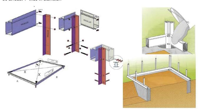
OPTION 2: Cutting the anchors and use concrete screws/self-tapping screws
